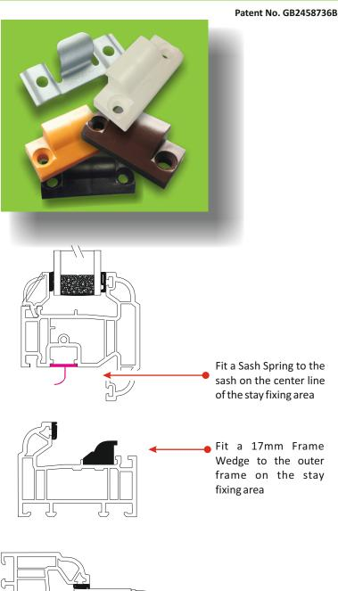
It may be necessary to pack the sash/glass at this point as shown
